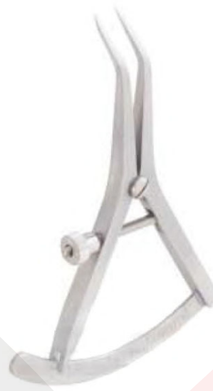
SM6-021 Measuring Loop angled length 9cm measuring range 0-40mm
